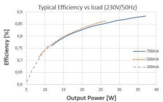
OTI DALI 35 NFC TW L Typical Efficiency vs. Load (230 V / 50 Hz)
